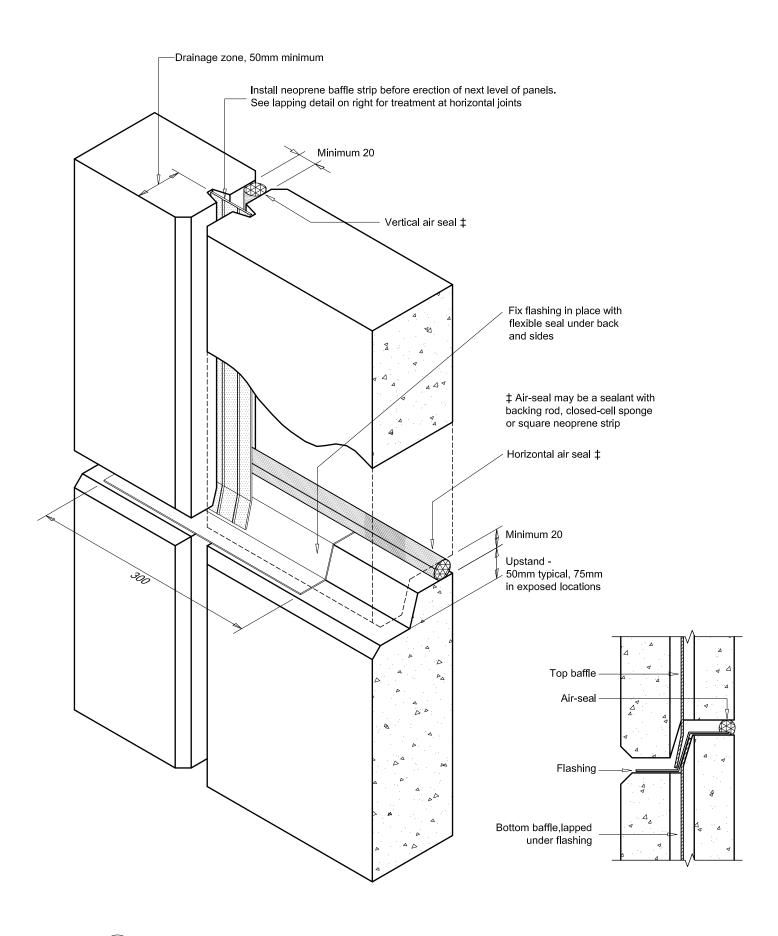
(C1) HIGH-RISE CONSTRUCTION, OPEN-DRAINED - CLADDING JOINT SYSTEM Scale 1:5
